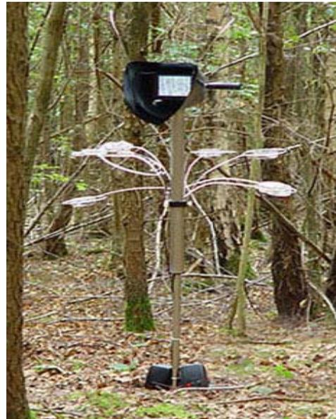
Figure 3: Periscope with screen and RF-tagged plates for triggering information displays
